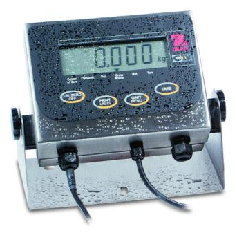
Combining the easy-to-use features of the popular Ohaus CD-11 indicator with a stainless steel washdown housing, the CW-11 provides an extremely durable indicator for industrial applications. Meeting NEMA 4X and IP-65 standards, the CW-11 can support up to four 350 ohm analog load cells for use in industrial and laboratory applications.
